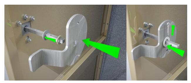
12. **Upper Lock Bar**: The lock bars can be attached at this point. Link the upper lock bar you slid into the door (step 12) to the CAM using (1) pan head screw (#10-24 x 1" zinc plated), (1) nylon washer (.5 OD x .266 ID x .06 THK, this get sandwiched between the CAM and lock bar), and (1) nulock nut.
