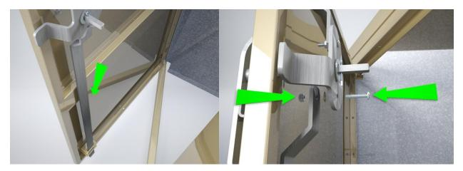
14. **Continue the Bank**: The rest of the bank can now be constructed, continue by locating another frame (remove the door and hinge) then attach it to a splice plate (just as you would a wall). Repeat this on the opposite end of the locker. A divider panel can now be added by following step 5 and the rest of the locker can be assembled by repeating steps 6-16. Finish the remaining lockers until you reach the end of the bank configuration (using a painted wall at the end).
