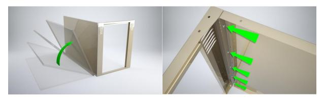
4. **Back Frame**: The back frame should be installed next. Repeat step one, removing the door and hinge from the frame. Stand up the frame and position it on the other end of the wall and attached it using (5) pan head screws. You should now have two frames and a wall standing ready for the divider panel.
