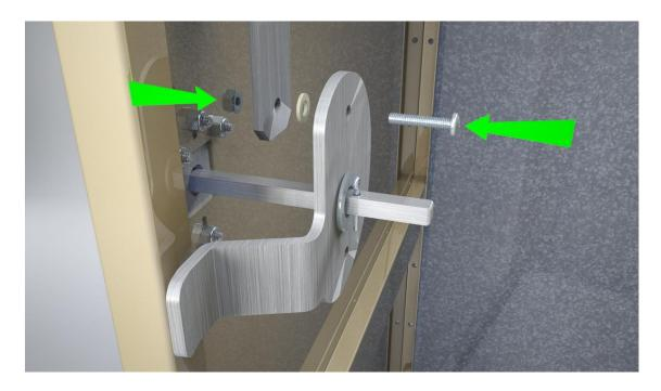
13. **Lower Lock Bar**: Now install the lower lock bar by sliding it through the guide on the bottom of the door then link it to the CAM using (1) pan head screws (#10-24 x 1" zinc plated), (1) nylon washer (.5 OD x .266 ID x .06 THK, these get sandwiched between the CAM and lock bar), and (1) nylock nut.
