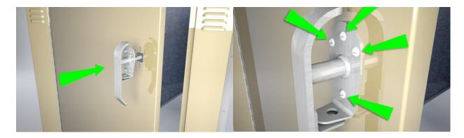
10. **Upper Lock Bar Prep**.: Now the CAM and lock bars can be installed. The upper lock bar must be inserted into the guide at the top of the door before the CAM can be installed.
