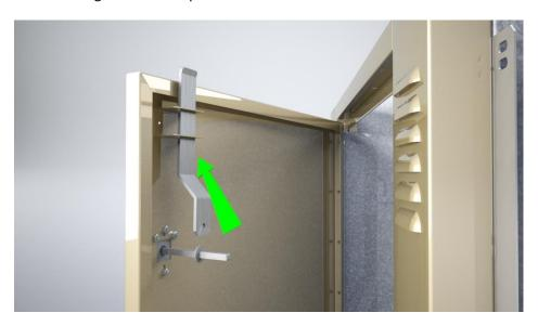
11. **Lock CAM**: The CAM slides onto the padlock handle shaft after a nylon washer (.75 OD x .50 ID x .06 THK), insure the orientation of the CAM is correct otherwise the unit won't lock properly. Next secure the CAM using a zinc washer (.438 ID x 1 OD x .083 THK) and cotter pin (bend the legs of the cotter pin once inserted to keep it snug).
