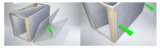
7. **Top**: The locker top can now be installed (we recommend using two people to carry these panels as they are very heavy) lift the top over the two frames, divider panel, and walls you have assembled in the previous steps. Slide a splice plate between the top and wall (this supports the top of the next locker in the bank). Now from inside the locker, attach the frames and walls to the top using (24) pan head screws, (6) for each wall and (6) for each frame.
