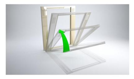
3. **Exterior Wall**: Next locate an exterior wall (these are painted/powder coated walls). Attach the wall to the frame using (5) pan head screws insuring the painted side faces the outside of the bank of lockers and is flush with the frame.
