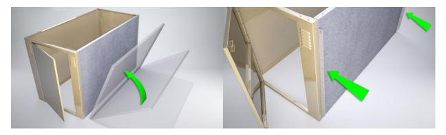
6. **Top**: The locker top can now be installed (we recommend using two people to carry these panels as they are very heavy) lift the top over the frame, back panel, and walls you have assembled in the previous steps. Slide a splice plate between the top and wall (this supports the top of the next locker in the bank). Now from inside the locker attach the frame, back panel, and walls to the top using (24) pan head screws; (6) for each wall, (6) for the frame and (6) for the back panel.
