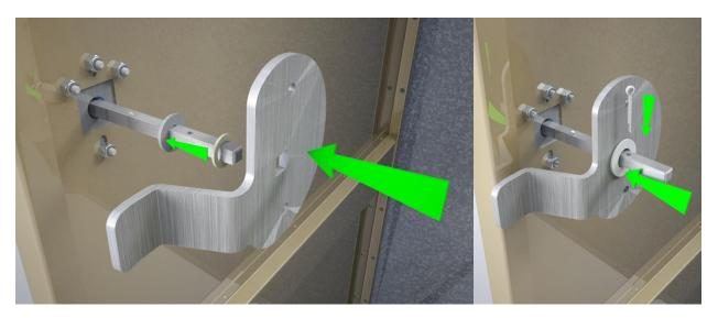
Upper Lock Bar: The lock bars can be attached at this point. Link the upper lock bar you slid into the door (step 12) to the CAM using (1) pan head screw (#10-24 x 1" zinc plated), (1) nylon washer (.5 OD x .266 ID x .06 THK, this get sandwiched between the CAM and lock bar), and (1) nylock nut.
