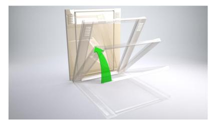
3. **Exterior Wall**: Next locate an exterior wall (these are painted/powder coated walls). Attach the wall to the frame using (5) pan head screws insuring the painted side faces the outside of the bank of lockers and is flush with the frame.
