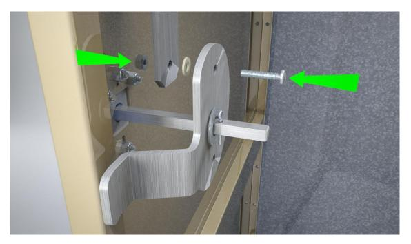
11. Lower Lock Bar: Now install the lower lock bar by sliding it through the guide on the bottom of the door then link it to the CAM using (1) pan head screws (#10-24 x 1" zinc plated), (1) nylon washer (.5 OD x .266 ID x .06 THK, these get sandwiched between the CAM and lock bar), and (1) nylock nut.
