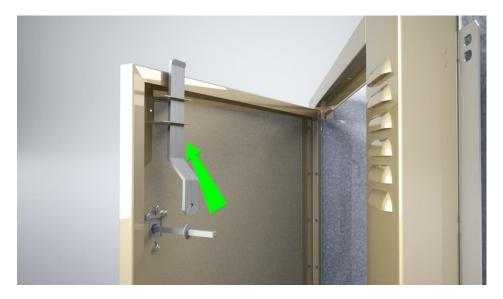
Lock CAM: The CAM slides onto the padlock handle shaft after a nylon washer (.75 OD x .50 ID x .06 THK), insure the orientation of the CAM is correct otherwise the unit won't lock properly. Next secure the CAM using a zinc washer (.438 ID x 1 OD x .083 THK) and cotter pin (bend the legs of the cotter pin once inserted to keep it snug).
