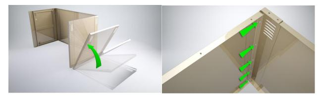
5. **Interior Wall**: Locate a galvanized (non-painted) interior wall. Position the wall between the frame and back panel you have already setup. Now insert a splice plate between the frame and wall (this links the lockers in the bank giving them more stability/rigidity) and secure the wall to the frame using (5) pan head screws. Next secure the wall to the back panel using (5) pan head screws, insuring both splice plates are aligned and sandwiched between the panels.
