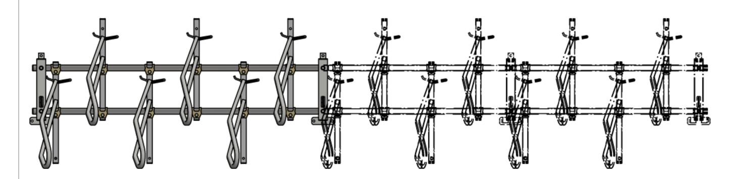
When daisychaining Vertical+ or Vertical No Scratch® rack modules, build each successive module so that the first bike support loop is height staggered relative to the adjacent loop in the prior module.
