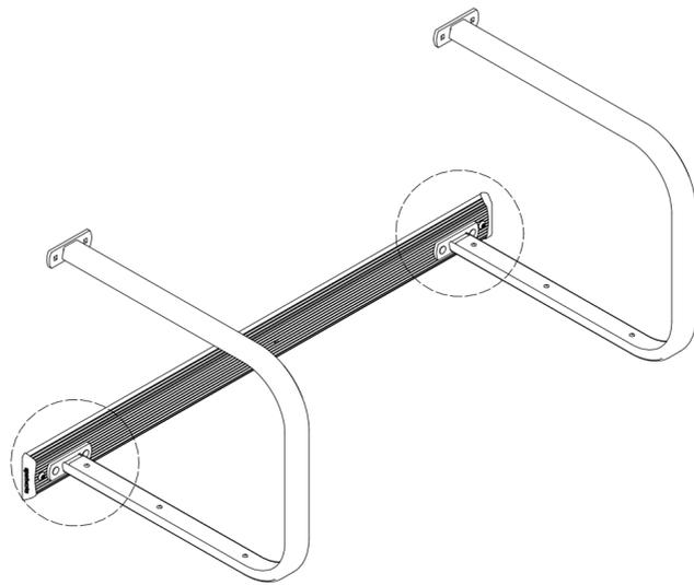
2. For the second rail, insert only one fastener in the outside hole of one of the rack feet as shown.
