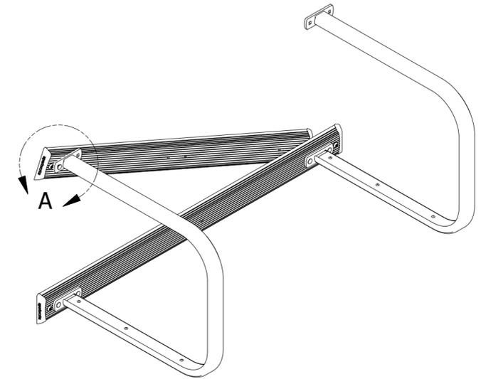
3. Rotate the opposite end of the rail up to the other bike rack foot and install all fasteners in both racks.
