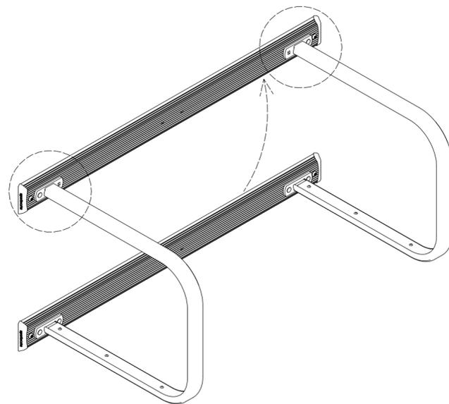
4. Install remaining racks and fasteners. Remove the endcap fasteners shown if rails are to be ground mounted. Ground anchors will retain endcaps. Tip assembly upright as shown.
