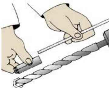
4. Before starting to drill the hole, it is important that eye and ear protection are used. Make sure the hammer drill is in the hammer mode and start drilling your hole. Continue drilling until the tape on the bit or the drill gauge meets the base material- this means that the required depth has been reached.
