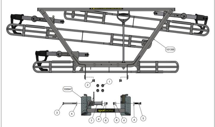
Note: Standoffs can shift during service because of impacts. When installing the Apex pivot plate on pre-installed standoffs, it may be necessary to loosen the standoffs from the back bumper structure in order to align them to the 14" and 18" hole pattern. Bolt the pivot plate to standoffs, and tighten standoff bolts.
