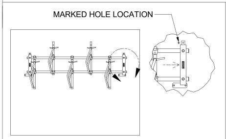
Slide the rack laterally to the left or right in order to get access to each marked hole location with a drill. Follow Step 2 of Section 3 to drill a 3/8" hole for each marked location.
