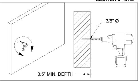
Using a hammer drill and a 3/8" carbide tipped hammer drill bit (following ANSI Standard B212.15) drill a hole on each of your installation marks.
