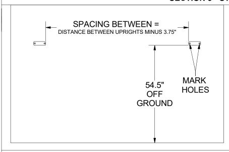
Determine the next wall mount bracket location by referring to the diagram to the left and the table in Step 8 of Section 2.
