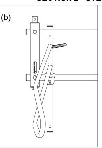
Install this first bicycle support in the low position about 2" to the right of the left hand upright. If you have the optional security cables for this rack, please refer to the assembly instructions that came with the security cables now.
