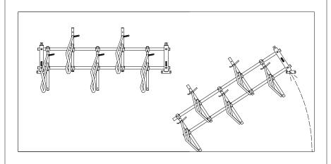
Lift up the side of the rack that is 10" beyond the free wall mount bracket by following Step 6 of Section 3.
