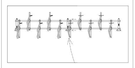
Lift up the other end of the rack and insert the cross-members into the upright. Ensure the cross-members are as far into the upright as they can go. Tighten both joints of this upright again.
