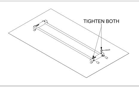
Insert opposite ends of cross-members into the second upright, then install end caps and tighten both joints.
