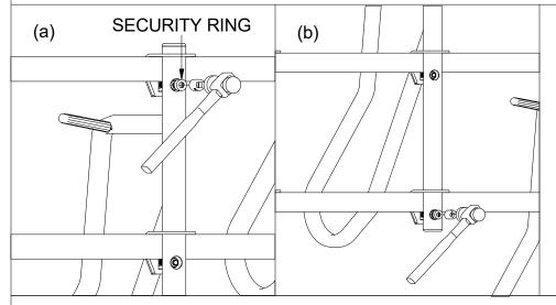
For **MEDIUM** security, use a 9/16" socket and a hammer to tap a security ring around the locking flanged hex nut of the upper clamp for each bicycle support in the lower position as shown in (a), and the lower clamp for each bicycle support in the upper position as shown in (b).
