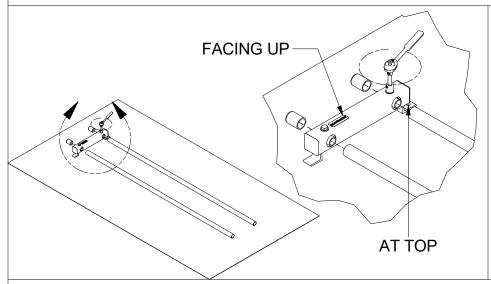
Place the next sections upright on the ground, face up as shown. Only one upright is required this time. Install both cross-members from the right hand side of the upright as shown. Then install the end caps from the left and tighten both joints.
