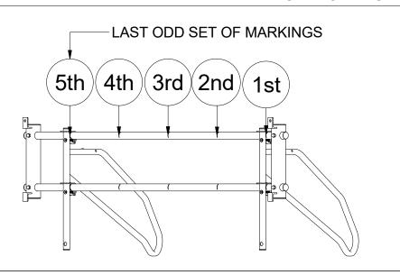
Align the left hand edge of the second bicycle supports rectangular tube with the last odd set of markings you made in Step 8 of Section 2.
