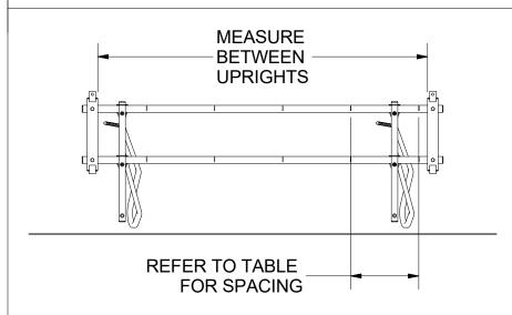
Mark the remaining bicycle support locations on the back of the cross-members by measuring from the first two 2" marks you made. Refer to the table below to determine the remaining bicycle support locations. Mark both cross-members for each bicycle support location.
