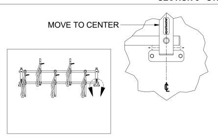
Center the upright laterally within the wall mount bracket as shown. To easier move the rack laterally, push the top of the rack towards the wall while pushing either to the left or to the right as required.
