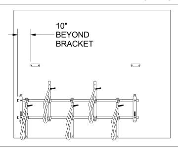
Position the assembled rack as close to the wall as possible for ease of mounting. Also, if possible position one end of the rack approximately 10" either to the left or right of one of the wall mount brackets.
