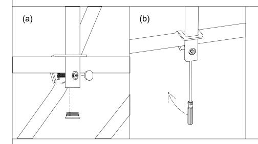
Start by removing the rectangular endcap in the end of the bike mount closest to the security ring and the round endcap hiding the security ring, as shown in (a).
