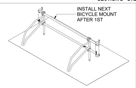
Starting back at the first bicycle support installed, install the next bicycle support (to the right of the first) in the upper position following Steps 14 through 16 of Section 2.
