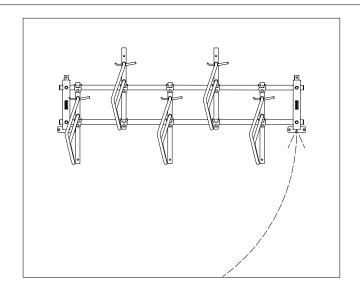
Lift up the opposite side of the rack, resting on the ground, and insert the lower L-bracket of the upright into the remaining wall mount bracket as shown.
