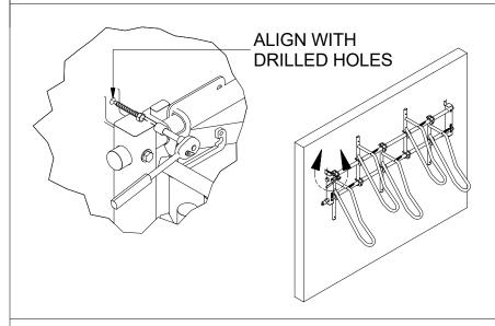
Slide the rack back so that the holes in the L-brackets in the uprights align with the drilled holes in the wall as shown. Insert a lag screw through one of the upright L-brackets and fasten it to the wall using a 9/16" wrench.
