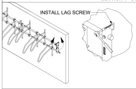
Bolt this upright to the wall by inserting a lag screw through the L-bracket and fastening it to the wall using a 9/16" wrench as shown.
