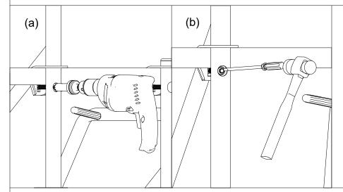
Start by removing the round endcap hiding the security ring.
