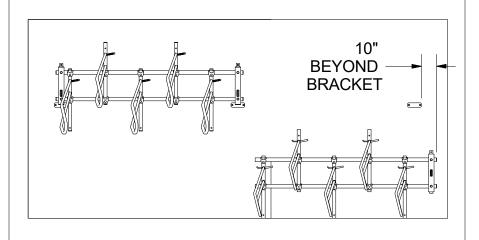
Position the assembled rack as close to the wall as possible for ease of mounting. Also, if possible position the end of the rack with the upright either 10" to the left or right of the free wall mount bracket.
