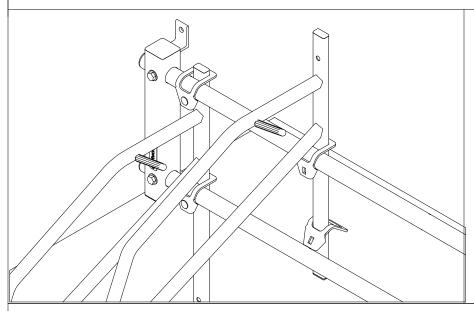
Position the second clamp by sliding up the rectangular tube. Push the lower portion of the rectangular tube back so the clamp can be hooked around the lower cross-member as shown. Then repeat Steps 3 and 4.
