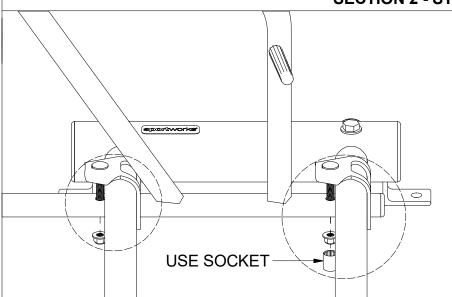
Using a 9/16" socket, place a locking flanged hex nut into the socket, then insert the nut through the corresponding hole in the back of the rectangular tube and thread the nut onto the carriage bolt. Repeat for the second carriage bolt. Thread the nuts until the locking portion of the nut is reached.
