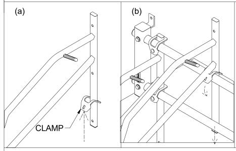
Slide a clamp up the rectangular tube as shown in (a), prior to installing this bicycle support in the upper position. Ensure the rectangular tube portion of the support is positioned behind the cross-members and hook the clamp over the top of the upper most cross-member as shown in (b).
