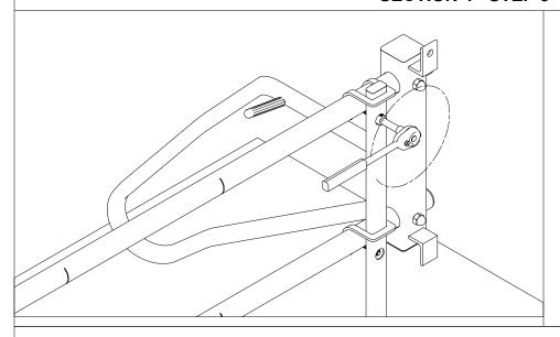
Tighten the first bicycle supports flanged hex nuts by following Step 11 of Section 2.
