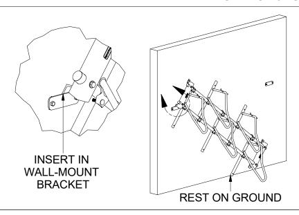
Lift up the side of the rack that is 10" beyond the wall mount bracket so the lower L-bracket of the upright can be inserted into the wall mount bracket as shown.
