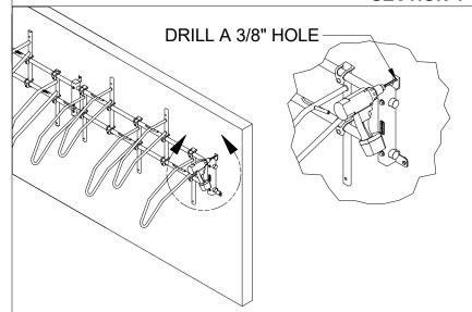
Push this new upright up against the wall and use the L-bracket as a guide to drill a 3/8" hole in the wall as shown.
