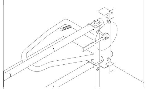
Using a 9/16" socket and ratchet, tighten the flanged hex nuts for both clamps on the installed bicycle supports.
