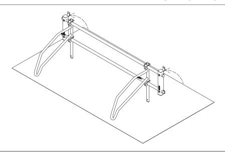
Now flip the assembly up so the uprights are oriented vertically and the assembly is resting on the bottom edges of the bike supports as shown. This will make installing the remaining bike supports easier
