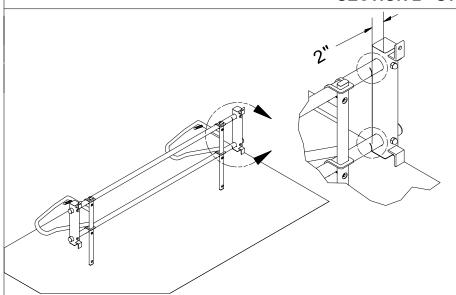
Mark the first bicycle support location on the back of both cross-members using a tape measure and a felt pen. Standing behind the cross-members, mark the first location 2" to the left of the inside edge of the right upright.
