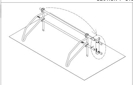
Remove the upright and end caps and install on the right hand side of the cross-members as shown.
