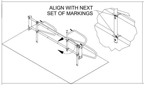
Align the left hand edge of the bicycle support's rectangular tube with the next set of markings you made in Step 8 of Section 2, then tighten both flanged hex nuts following Step 11 of Section 2.
