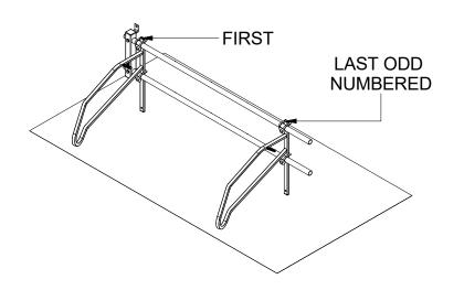
Install the first and last odd bicycle supports on the cross-members following Steps 1 through 5 of Section 2.
