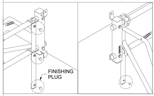
Install larger finishing plugs in all three holes in the back of each bicycle support as shown in (a).
