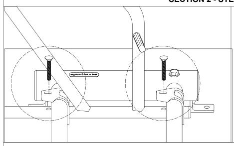
Place a carriage bolt through each of the square slotted holes in the front of the two clamps and into the corresponding holes in the front of the vertical tube of the bicycle support as shown.
