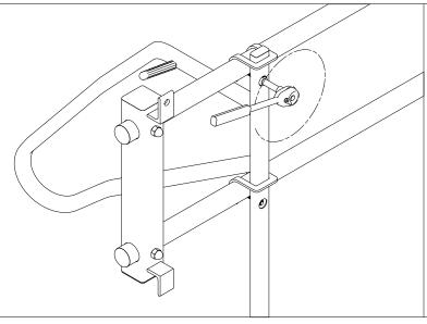
Tighten the last odd bicycle supports flanged hex nuts by following Step 11 of Section 2.
