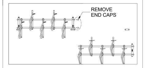
Before installing this next section to the wall, determine which side this section will be joined to the last.
