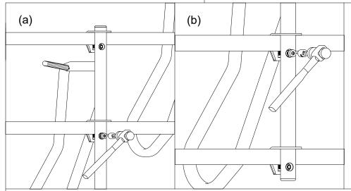
For **HIGH** security, use a 9/16" socket and a hammer to tap a security ring around the locking flanged hex nut of the lower clamp for each bicycle support in the lower position as shown in (a), and the upper clamp for each bicycle support in the upper position as shown in (b).
