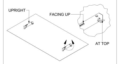
Place both uprights on the floor as shown approximately the width of the cross-members apart. Ensure the Sportworks decals are facing up and the L-brackets with the holes are at the top.
