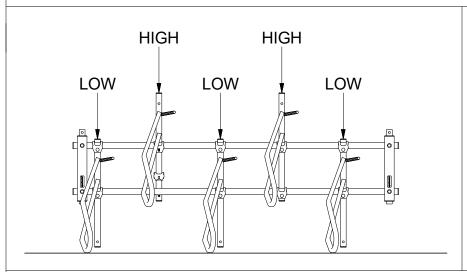
Continue installing the remaining bicycle supports ensuring each is alternating in height (low, high, low, high, etc.).
