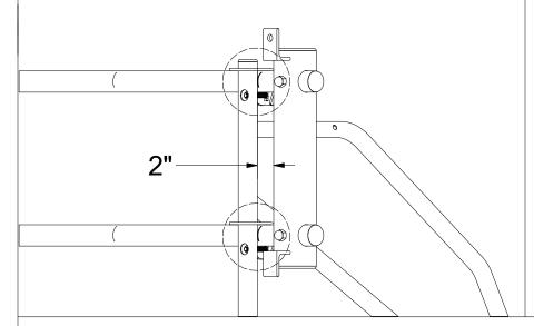
Align the left hand edge of the first bicycle support's rectangular tube with the first two marks you made in Step 7 of Section 2.
