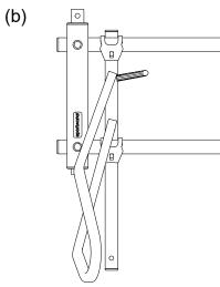
Position the second clamp by sliding down the rectangular tube and around the upper cross-member as shown in (a). Let clamp rest around the cross-member as shown in (b).
