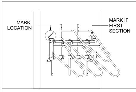
Once the upright has been centered with the wall mount bracket, push the rack up against the wall and mark the mounting hole location through the upper L-bracket of the upright as shown.
