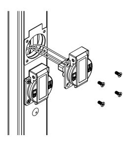
Connect power, neutral, and ground wires from conduit to GFCI circuit breaker (receptacles are rated for 125V/15A max).
